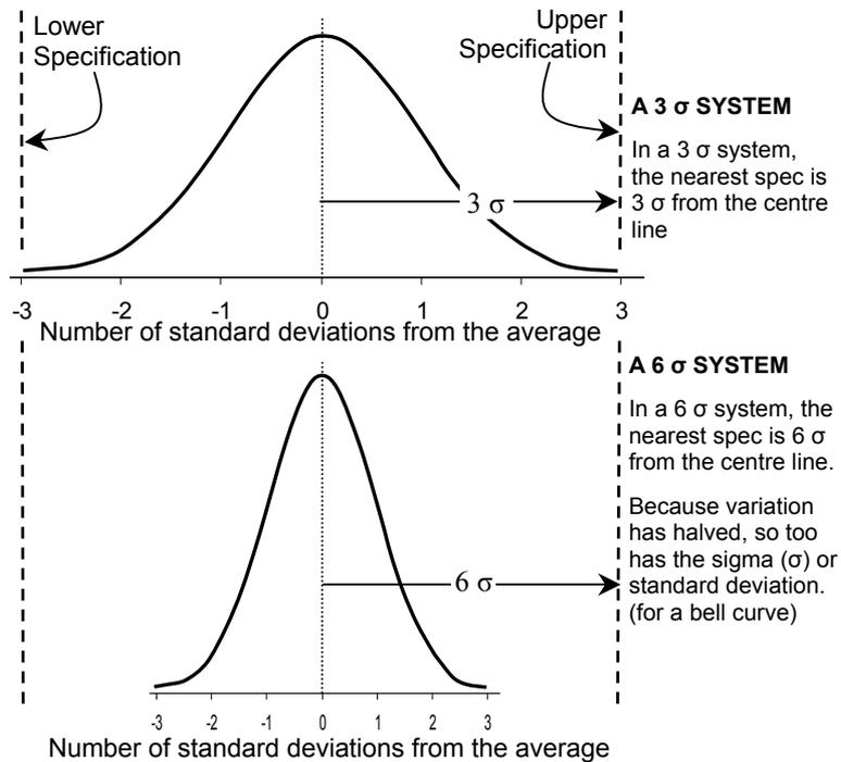
This, then, is the origin of the term six sigma. <sup>(3)</sup> In a six sigma system, every part and every processing step shows variation such that the nearest specification is six sigma away. If the distribution is correctly centred and bell shaped, it must display no more than half the variation allowed by the specifications to be a six sigma system. Nevertheless, many people are inclined to ask why one would bother to reduce variation so far below the specified requirements.
